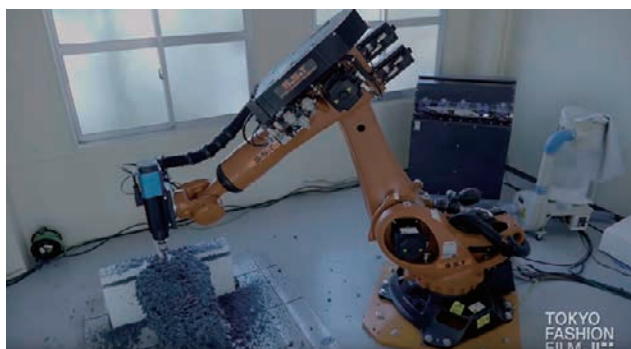
Fig. 2 Shaving a roll of cloth with a robot arm. Courtesy of noiz
